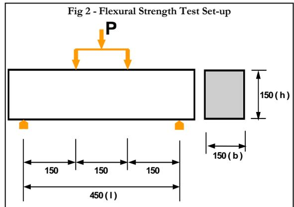
USA Standard C1018 and Japanese Standard JCI-SF4 are both based on the third point loading of a beam of square cross section spanning a three times its depth (Fig. 2).
