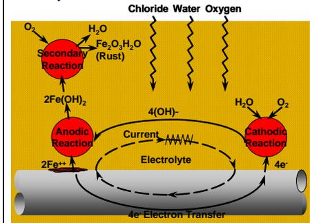
Figure 3 - Design model based on key corrosion mechanisms.  $T_0$  is the time taken for chlorides to reach the steel and  $T_1$  is the time taken to form sufficient corrosion product to cause spalling. Use of CSF extends both timeframes
