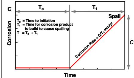
Figure 4 - Silica fume concrete (ref Gautfall 1986) has a chloride diffusion coefficient 5-10 time lower than an OPC concrete. This increases the time to activation ( $T_0$ ) by 5-10 times
